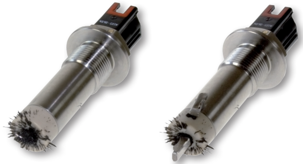
Channel 1: Fine Fine metal particle build-up
